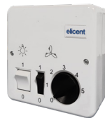
RVS/L 5 speed controller with on/off and light switch. Max load 0,5 A. IP42 protection. Size 118x118x58 mm.
