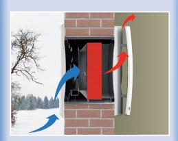
REC Duo 100 is a "push-pull" HRU with reverse flow. It is provided with a ceramic heat exchanger that accumulates the heat from the extracted air during the "pull" cycle and releases it to the new fresh air during the "push" cycle.
