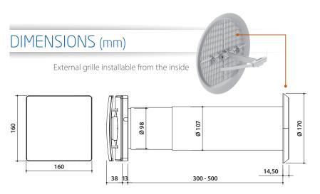
For walls with thickness > 500 mm: It is necessary to use the telescopic duct available as accessory
