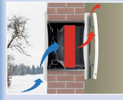
REC Duo 100 is a "push-pull" HRU with reverse flow. It is provided with a ceramic heat exchanger that accumulates the heat from the extracted air during the "pull" cycle and releases it to the new fresh air during the "push" cycle.
