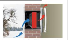
REC Duo 100 is a "push-pull" HRU with reverse flow. It is provided with a ceramic heat exchanger that accumulates the heat from the extracted air during the "pull" cycle and releases it to the new fresh air during the "push" cycle.
