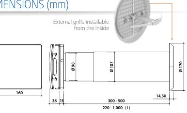
(I) For walls with thickness > 500 mm: It is necessary to use the telescopic duct
