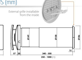
(I) For walls with thickness > 500 mm: It is necessary to use the telescopic duct
