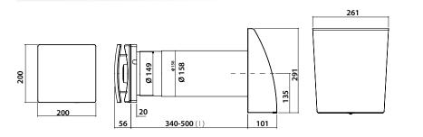
(I) For walls with thickness > 500 mm: It is necessary to use the telescopic duct available as accessory Cod. 2KT0015
